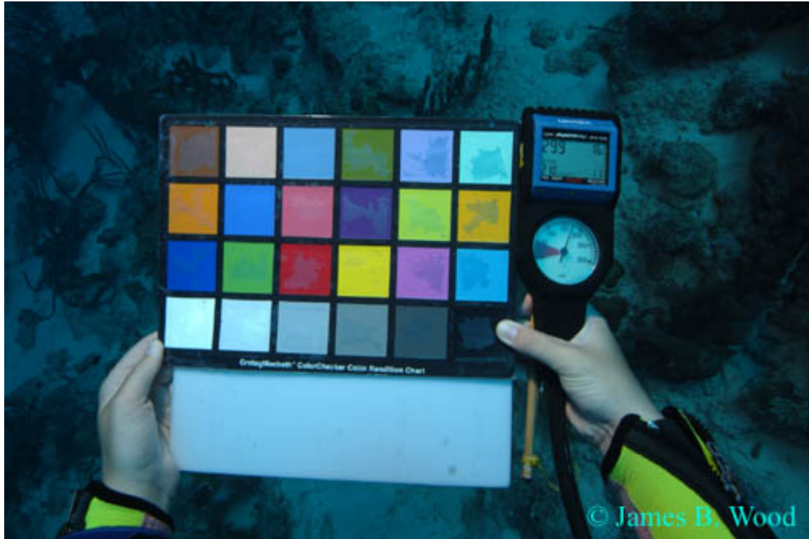
Figure 14. Macbeth color card at a depth of 30 meters. This photograph was taken with dual underwater strobes (flashes).
